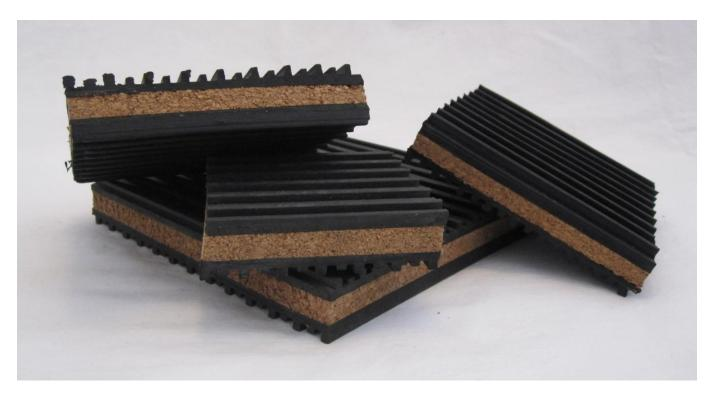
Rubber Cork Pads are designed to reduce problems in industry caused by vibrations and structure borne noise. Cork with ribbed pads on either side provides additional isolation and positive grip.
